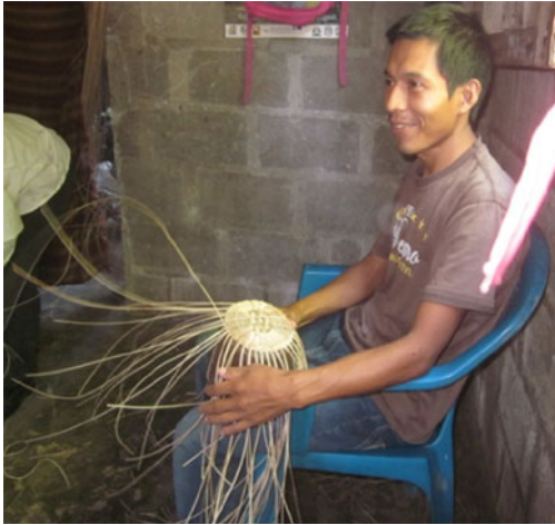
Fig. 1. Elaboration of Monstera maderaverde (“mimbre”) hat on a wooden mold.
